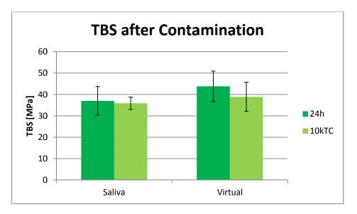
Fig. 16: Tensile bond strength of Monobond Etch & Prime / Variolink Esthetic on IPS e.max CAD samples after contamination with saliva and Virtual Extra Light Body respectively
