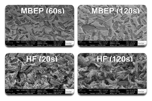
Fig. 14: SEM images of IPS e.max CAD surfaces after varying lengths of contact time with 5% hydrofluoric acid (HF) and Monobond Etch & Prime (MBEP)
