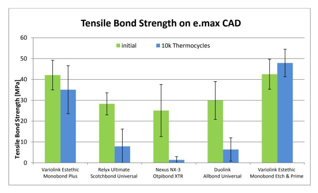
Fig. 10: Tensile bond strength of various adhesives and primers on IPS e.max CAD
