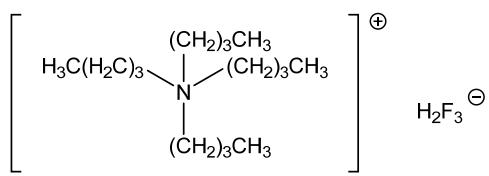
Fig. 5: Structure of Ammonium polyfluoride
