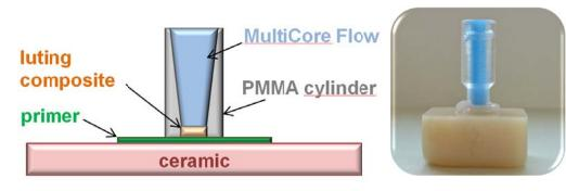
Fig. 7: Test specimen for tensile strength testing
