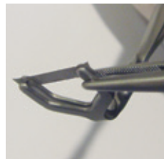
5 Use hemostat or pliers to (gently) clamp down on one prong and make sure the pin has penetrated the strip on that side only
