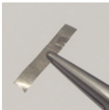
1 Cut a 1" length of strip and secure midway with a hemostat or pliers
