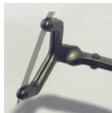
8 Notice fully closed, locked and penetrated strip (on both sides)
